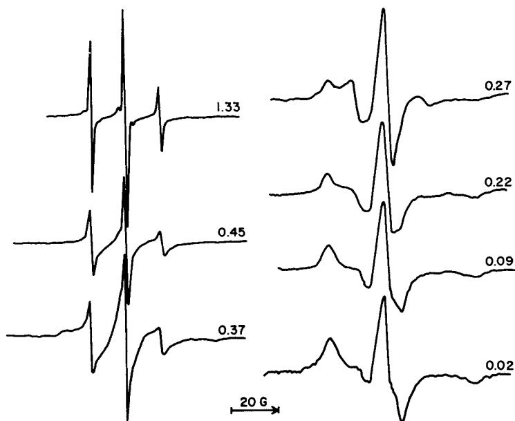
Figure 4. ESR spectra of Tempone noncovalently bound to lysozyme (mole fraction of Tempone, 0.018) at hydration levels of 0.02–1.33 g of water per gram of protein. All measurements were at 24°C.
